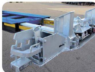
Option: Extension Front front load container 45' and swap within the legal maximum allowed (without special permit to transport). Neck height of 150 mm. Sliding extension guided by bearings and Teflon plates. Galvanized complete set extension to ensure their conservation.
