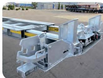
**Option 1:** front extension for 45' container loading within legal maximum length (without special transport permits)
