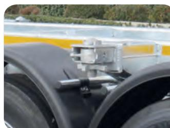
**Option 2:** extra twist locks in front part for advanced 20' container, to increase adherence in traction motor.
